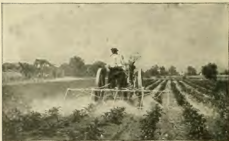
FIG. 41.—Row sprayer applying arsenate of lead to potatoes, showing arrangement of nozzles to cover vines. (After Britton.)
